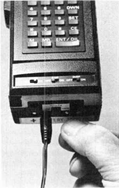
12-12. A small wall-type charger can be plugged into the bottom of the transceiver case. A full charge takes 14 hours.
