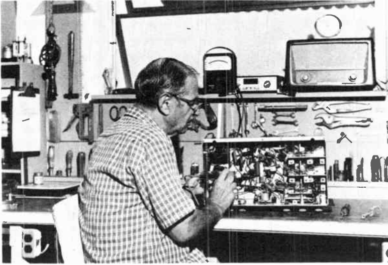
8-1. The basement workbench that is almost a standard fixture in American homes is ideally suited for ham radio and other electronic construction projects. Note wall-mounted tools, within easy reach.
