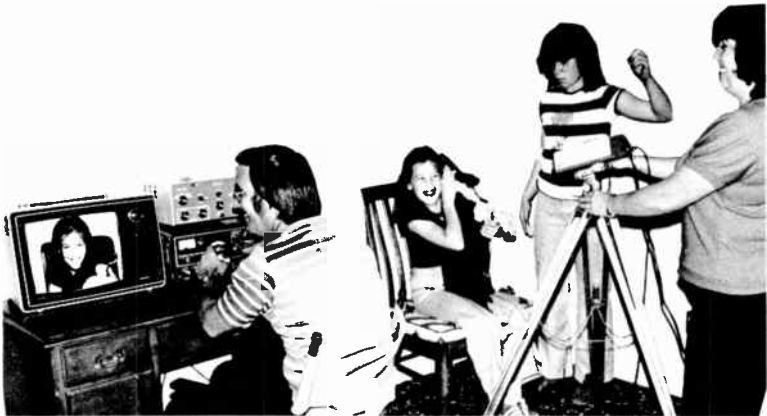
14-3. The whole family gets into the act when the ham shack becomes a two-television studio. SSTV converter is on top of transceiver on table. Monitor/receiver is at left.
