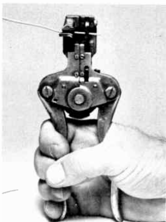
8-16. A wire stripper is a great time-saver. In this first step, the insulated wire is in the closed jaws, but the handles are open.
