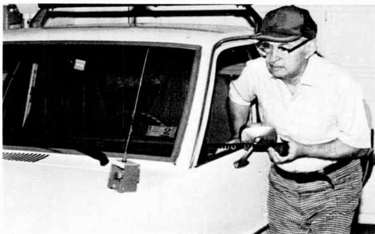
12-16. (above) Mobile antenna made from unfolded coat hanger is in ideal location on top of car on one arm of luggage rack. 12-17. (below) Cut-and-try method of pruning wire with aid of field strength meter (on fender) is quick and effective.
