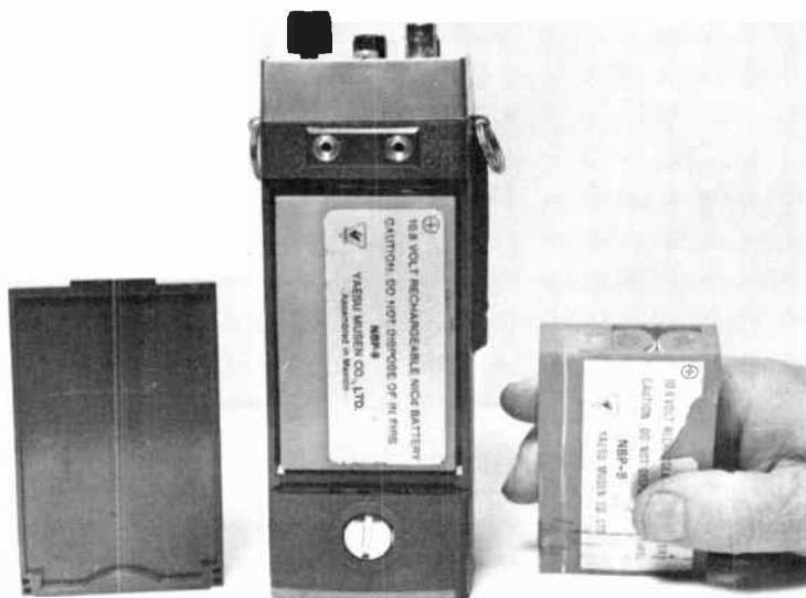
12-8. Flat-pack NiCad battery of 10.8 volts is standard with most HT's. Spare battery, at right, has opening in right corner for contact springs inside the case of the set.
