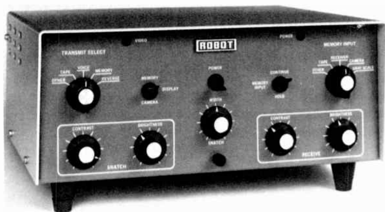
14-1. The Robot SSTV Scan Converter is popular with slow scan experimenters. It functions on both transmit and receive.
