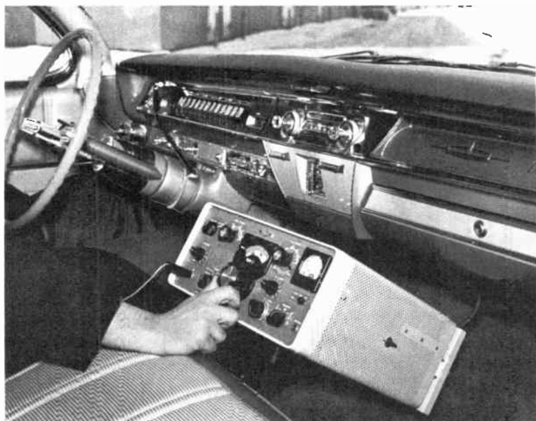
18-1. This large Collins KWM-2 transceiver, of the conventional tube type, mounts to a special plug-in base fastened to the floor of the car. Its current drain on the car's battery is considerable.
