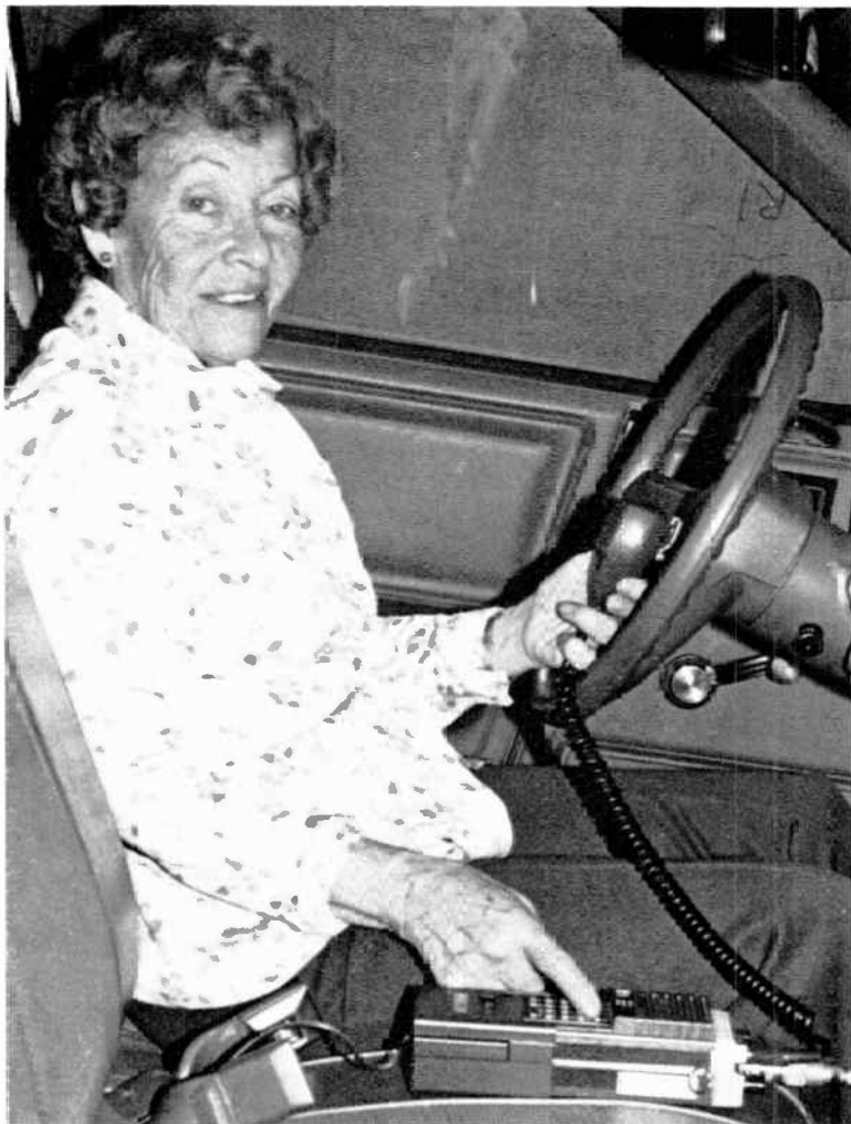
12-19. Handy-talkie is handy to operate in a car. It plugs into a battery adapter (under hand in photo) and connects to roof antenna by coax at extreme right. If passenger is to use rig at times, it can be pushed along the seat without disturbing any of the connections.
