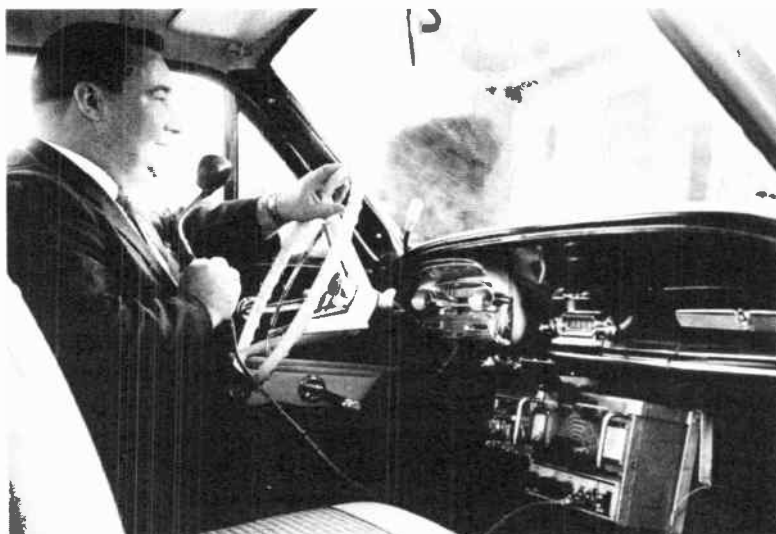
18-5. A telephone operator's chest-type microphone lends itself to mobile use because it remains in correct speaking distance from the driver's mouth. He presses switch on the mike's base to actuate the transmitter under the dash. Receiver is farther to left.
