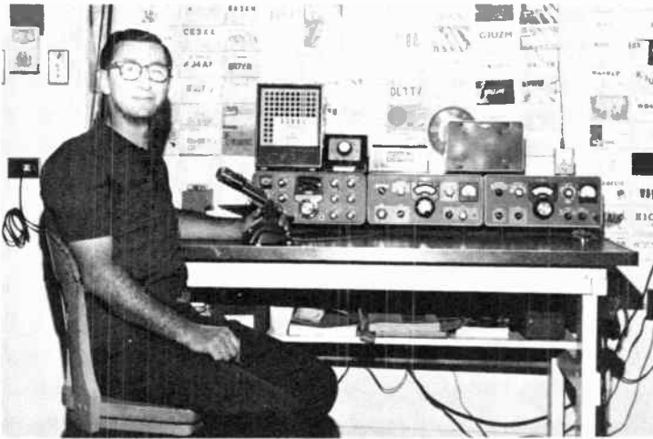
16-1. This spacious operating table in the basement shack of Paul Hertzberg, K2DUX, is a common door, sanded smooth and varnished. The support is made of 2 \times 3 " lumber, with a shelf to hold magazines, call books, etc. Note the wall plastered with acknowledgement cards from stations all over the world that Paul has worked with: Heath SB-110, at left, and Collins "S" Line, two units at right.
