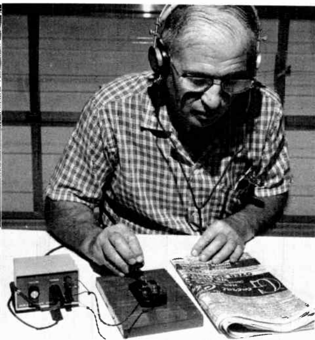
10-5. Key is mounted on board to keep it steady. Note student's arm full length on table, two fingers on key. Earphones are plugged into oscillator for private listening. Newspaper provides endless "copy" for practice sending.
