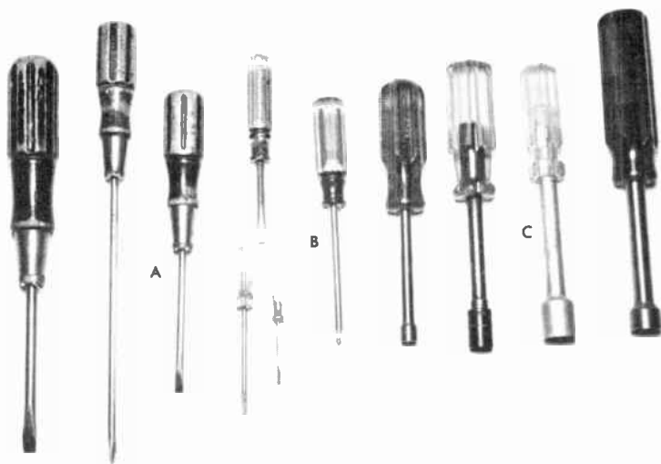
8-3. Tools for radio construction: (A) six sizes of screwdrivers, (B) Phillips-head screwdriver, and (C) four sizes of hex-nut drivers.
