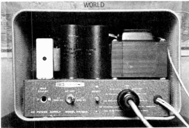
13-18. Surprise! The AC power unit is stowed neatly inside the loudspeaker cabinet, with its controls facing outward for easy adjustment.
