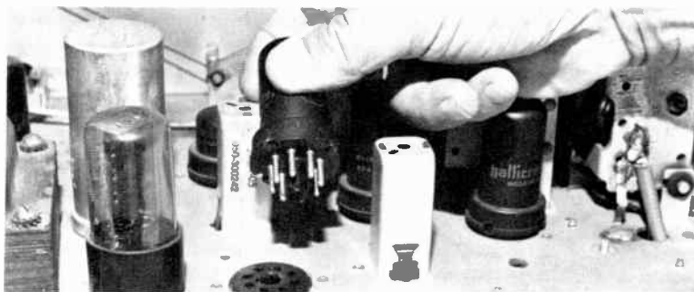
3-10. Then grasp the top of the tube firmly with dry fingers, pull without turning, and it will pop up without damage.
