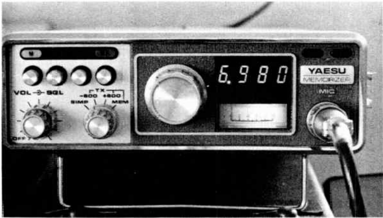
12-24. Four-digit frequency readout changes as the large center knob is turned. Push buttons at top left control memories, frequency split, tone squelch. Front of case is raised by U-shaped stand to allow voice from loudspeaker to come out.
