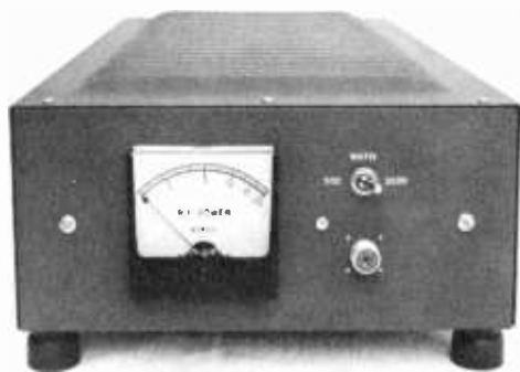
Figure 7. 2-KILOWATT DUMMY LOAD FOR 3-30 MC.
