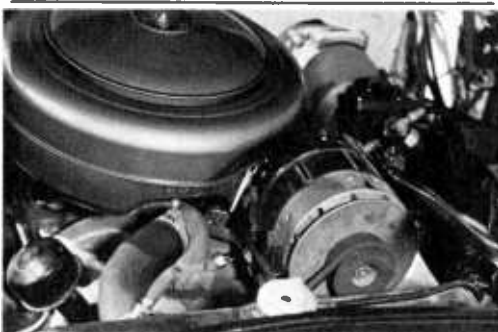
Figure 4 LEECE-NEVILLE 3-PHASE ALTERNATOR IS ENGINE DRIVEN BY AUXILIARY FAN BELT.
