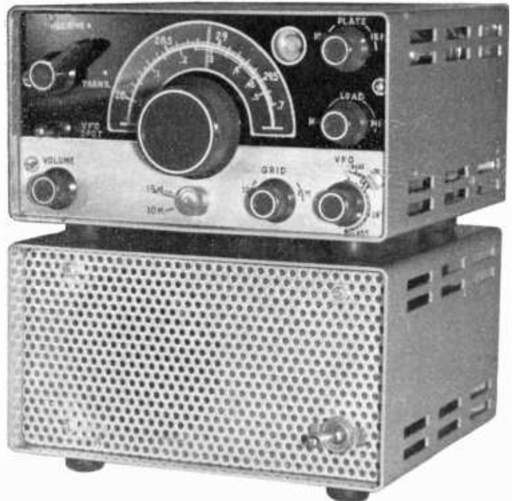
Figure 20 HOME MADE POWER SUPPLY FOR TRANSCEIVER FITS IN MATCHING CABINET WITH SPEAKER
