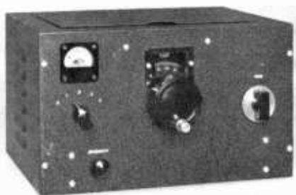
Figure 43 ANTENNA TUNER IS HOUSED IN METAL CABINET 7" x 8" IN SIZE.
