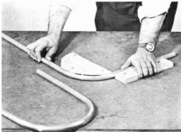
Figure 3 SOFT ALUMINUM TUBING MAY BE BENT AROUND WOODEN FORM BLOCKS. TO PREVENT THE TUBE FROM COLLAPSING ON SHARP BENDS, IT IS PACKED WITH WET SAND.
