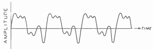
Figure 3 THE COMPLEX SOUND OF A MUSICAL INSTRUMENT IS A COMBINATION OF SIMPLE SINE-WAVE SOUNDS, CALLED HARMONICS. THE SOUND OF LOWEST FREQUENCY IS TERMED THE FUNDAMENTAL. THE COMPLEX VIBRATION OF A CLARINET REED PRODUCES A SOUND SUCH AS SHOWN ABOVE.
