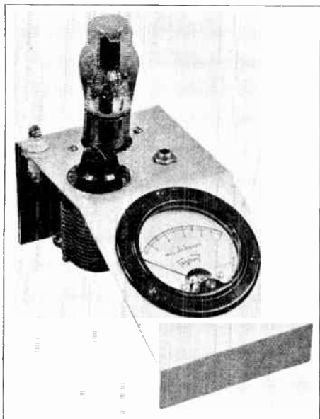
Fig. 18—A Piece of No. 12 Gauge Aluminum Is Bent in One Piece to Provide a Mounting Stand for the Overmodulation Indicator
