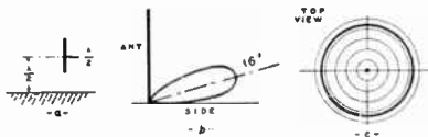
Half Wave Antenna, Same Height as Full Wave Antenna Above. Here the Radiation is Known as 16-Degree "Low Angle" Radiation.
