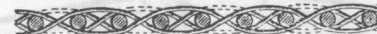
Fig. 15.—Plan view of the first four turns of a double basket coil.
