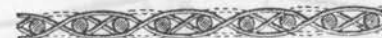
Fig. 15.—Plan view of the first four turns of a double basket coil.
