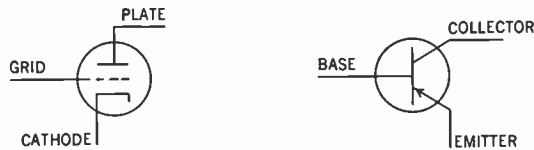
FIG. 14. Comparable elements in tubes and transistors: grid-base, cathode-emitter, plate-collector.
