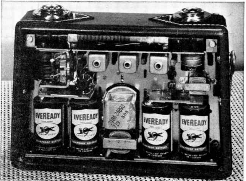
FIG. 14. A rear view of the Raytheon portable transistor receiver whose diagram appears in Fig. 12. (Courtesy Raytheon Mfg. Co.)
