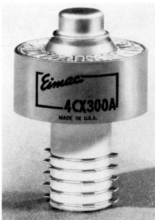
Figure 14.1(b). Ceramic power tetrode 4CX300A, using Design A approach, Maximum plate dissipation 300 watts at 500 MC. Maximum operating temperature 250°C. (Courtesy Eitel McCullough, Inc.)
