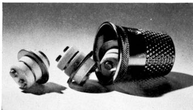
Figure 14.1(d). G.E. Type 7077. (Registered Type Number; first ceramic receiving tube in regular production (1959)). (Courtesy Receiving Tube Department, General Electric Company.)
