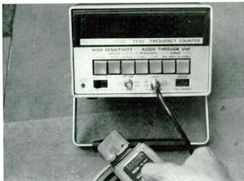
Fig. 1-56. Sencore FC45 frequency counter that is an excellent aid for VCR troubleshooting.
