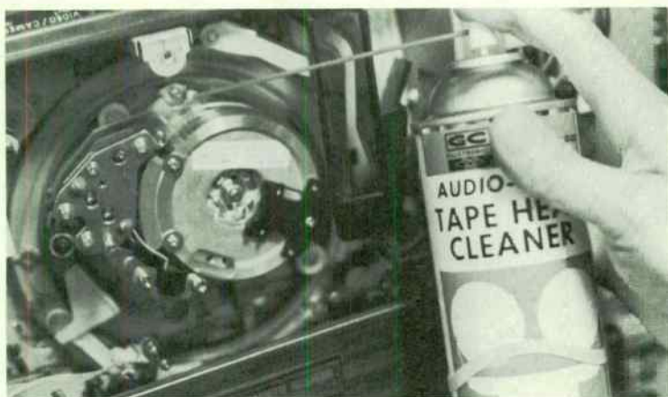
Fig. 7-8. Spray type head cleaner being used.
