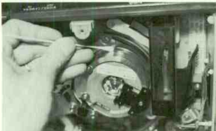
Fig. 7-4. Do not use cotton swabs for cleaning heads.
