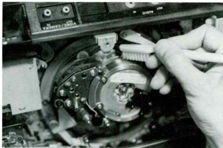
Fig. 7-6. A toothbrush can be used for cleaning clogged heads.
