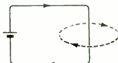
Fig. 4.5—An electric current and the magnetic flux set up thereby are linked with one another as indicated in this diagram, which shows the relative directions established by convention
