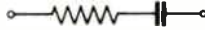
Fig. 24.4—Simple combination of circuit elements used as a starting point for study of two alternative approaches to signals
