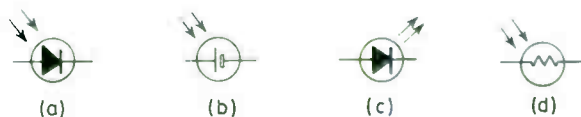
Fig. 10.18—Symbols for (a) photodiode, (b) photovoltaic diode, (c) light-emitting diode, and (d) photoconductive cell
