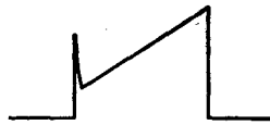
FIG. 21-14. The use of a narrow spike to aid in starting a linear-sweep current.
