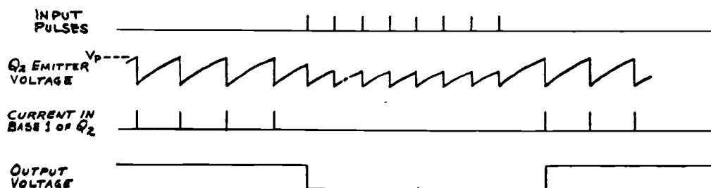
Pulse detection uses unijunction transistor as relaxation oscillator.
