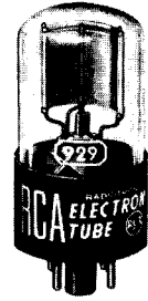
Fig. 24. A typical phototube. (Courtesy Radio Corporation of America.)
