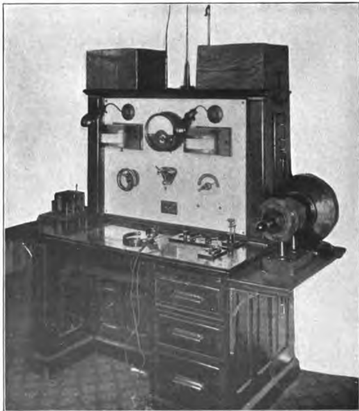
FIG. 20.—WIRELESS OPERATOR'S DESK, SIGNAL CORPS U. S. A.
