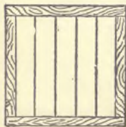
FIG. 32.—POLARIZER FOR ELECTRIC WAVES.
