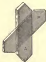
FIG. 18.—TOURMALINE PLATES CROSSED AT 45^\circ .
