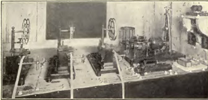
FIG. 308.—BULL SYNCHRONIZED SYSTEM. THE COLLECTORS.
