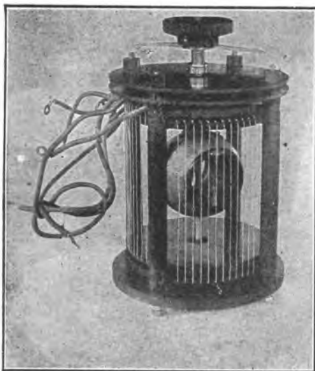
FIG. 259. The Marconi radiogoniometer—a radio instrument for locating the direction of a sending station.
