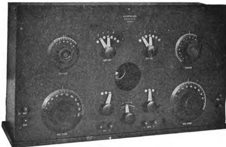
FIG. 207a. Grebe type C R 7 long wave receiving set. Range 500 to 20,000 meters.
