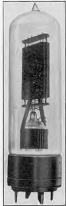
FIG. 137.—Western Electric Type Power Tube. Length: 30 cms.
