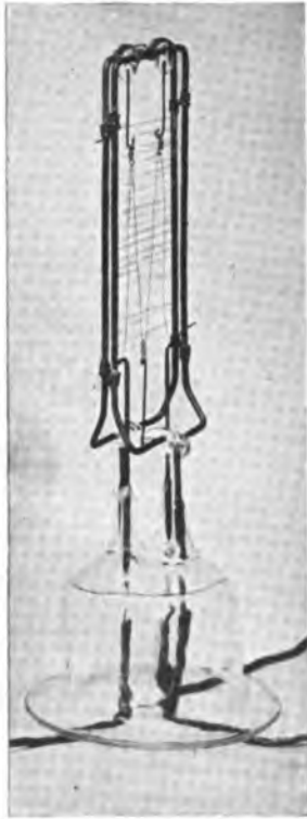
FIGURE 90—Filament and grid element of pilotron.
