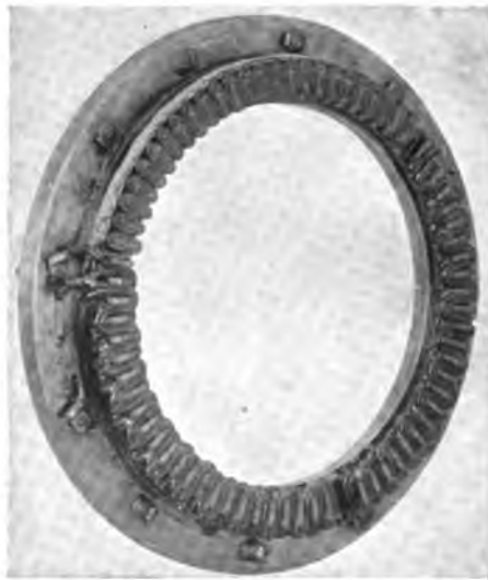
FIGURE 189—General Electric Company— Alexanderson telephone control relay; stator (field and armature).
