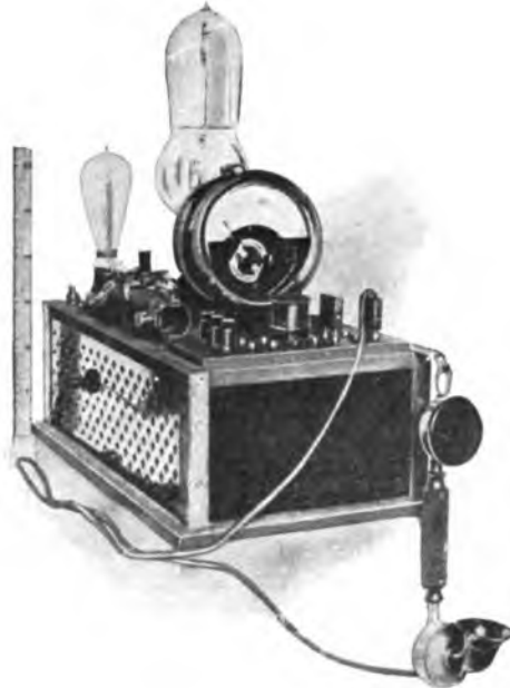
FIGURE 151—Telefunken Company-Meissner radiophone transmitter, 1913.
