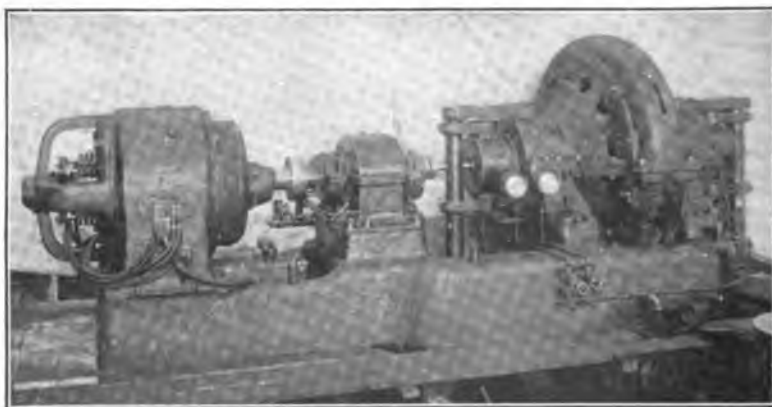
FIGURE 124—50 kilowatt, 50,000 cycle, General Electric Company-Alexanderson alternator.
