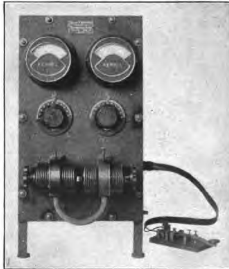
FIGURE 51—Front view. 0.25 k.w. Chaffee gap set. Designed by Cutting and Washington.
