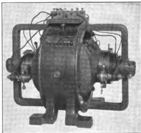
FIGURE 58—100-to-500 volt direct current rotary converter of T. Y. K. radiophone transmitter.
