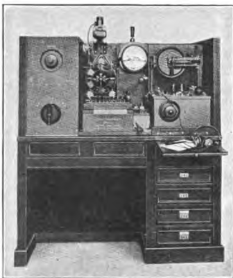
FIGURE 43—Lorenz Company "multitone" ship set.
