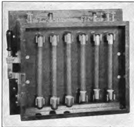
FIGURE 58—100-to-500-volt direct current coils for direct current supply circuit of T. Y. K. radiophone transmitter.
