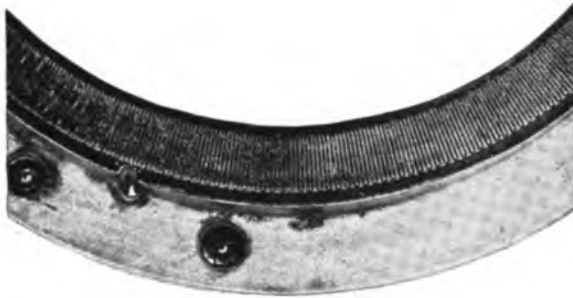
FIGURE 117—Portion of armature winding of 100,000 cycle Alexanderson alternator; 600-slot type.
