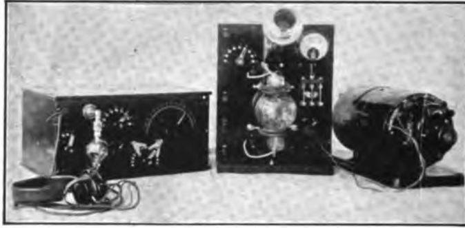
FIGURE 162—de Forest oscillon radiophone and radio telegraph transmitter and receiver (Type OJ3).
