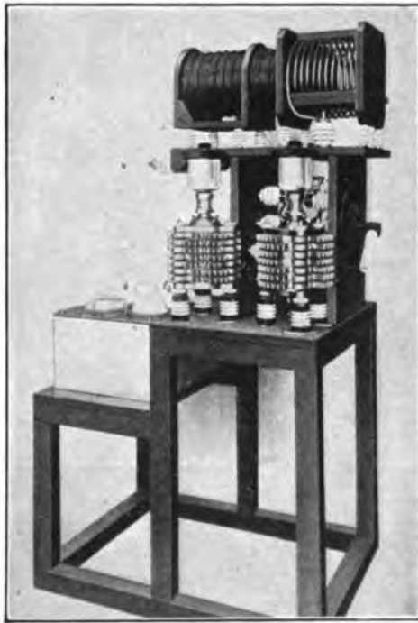
FIGURE 44—Lorenz Company "multitone" semi-high power set.
