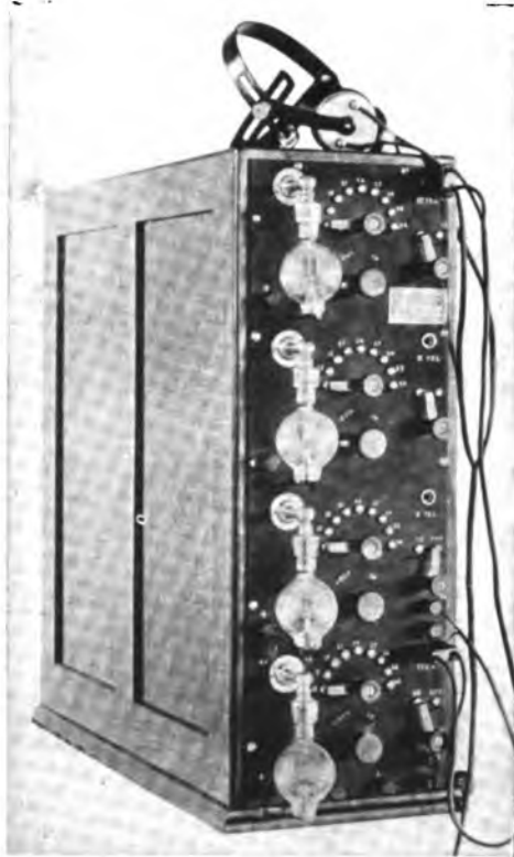
FIGURE 207—de Forest audion and three stage amplifier.
