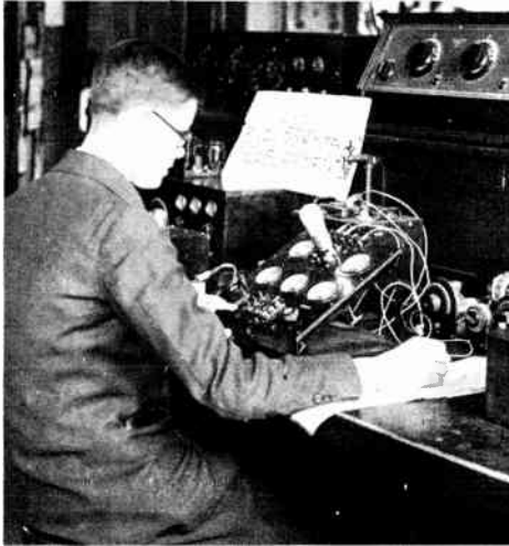
Fig. 204—Left: Laboratory type tube tester for taking tube characteristics. Right: How \mu is determined from the Eg- I_p characteristic curves for two values of plate voltage.
