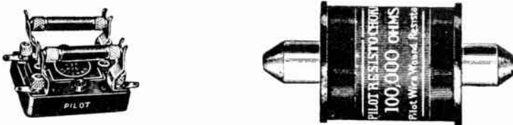
Fig. 315—Left: Resistance-coupling unit containing the plate and grid circuit resistors and the blocking condenser for a single amplifier stage. Right: Wire-wound form of plate resistor with special end terminals to snap in place in the unit at the left.
