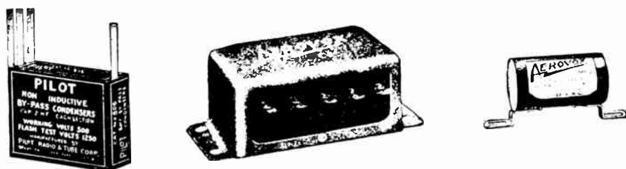
Fig. 276—Several by-pass condensers used in radio receivers. Left: 3-section condenser, each section is .2 mf. Middle: 4-section condenser with common terminal. Right: Compact, tubular form of by-pass condenser made in sizes from .01 to .1 mf.
