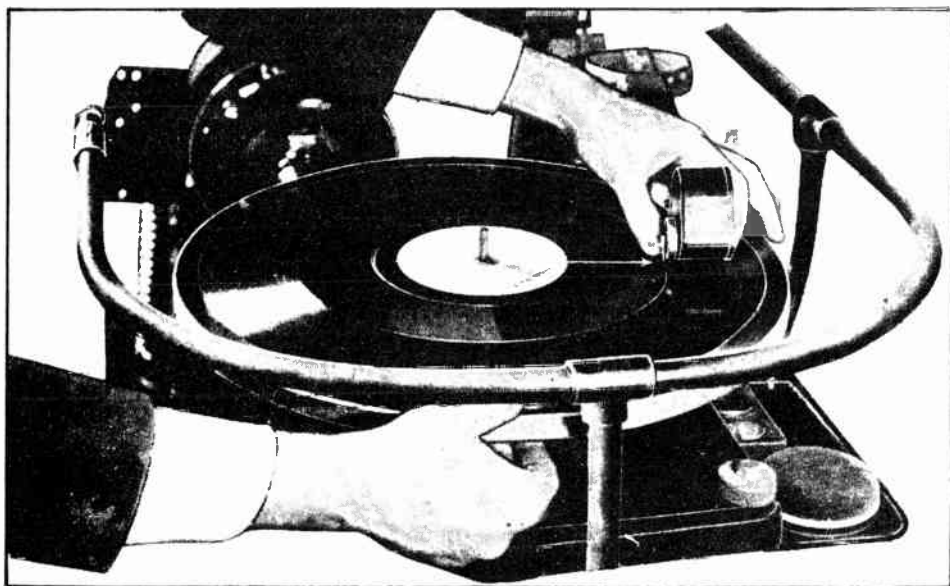
Fig. 489—The method of setting the record at the "starting point" in the sound-on-disc system. The needle of the phonograph pickup unit is placed in the starting mark on the disc.
