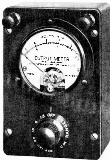
Fig. 153—Left: Copper-oxide rectifier type output meter with 4000 ohm input impedance arranged for radio receiver testing.
