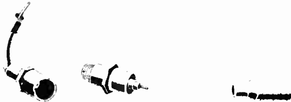
Fig. 400—From left to right are shown the gooseneck and metal shield cap, shielded spark plug, spring, and special hollow insulating sleeve which are used in the shielding arrangement of Fig. 399.
