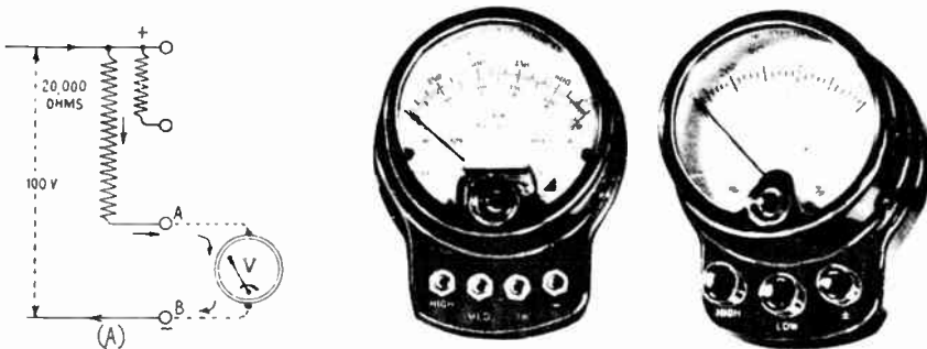
Fig. 144—(A) Connection of a voltmeter to the output circuit of a B-eliminator. Middle: A 3-range d-c high resistance voltmeter having a resistance of 1000 ohms per volt. Right: A 2-range a-c voltmeter. These instruments are very useful in radio tests and service work.
