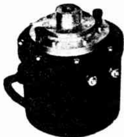
Fig. 420—Left: Typical electro-dynamic driving unit for an air-column type loud speaker. Right: An exciter unit for supplying low-voltage direct current for the field of the speaker unit at the left. The exciter operates from the 110 volt a-c line and contains a suitable transformer and rectifier bulb.
