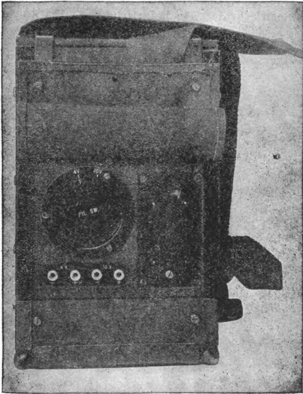
Fig. 31. Illustrating the key, in closed position, and the filament switch.
