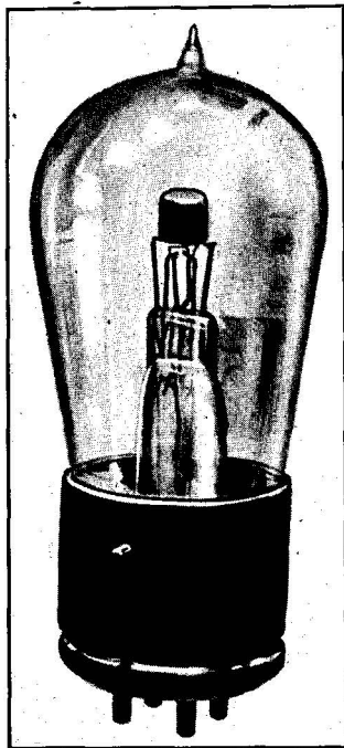
FIG. 130.—General Electric type Receiving Tube. Length: 10 cms.
