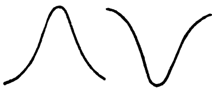
Figs. 85 and 86.—H.F. response curve inversion.
