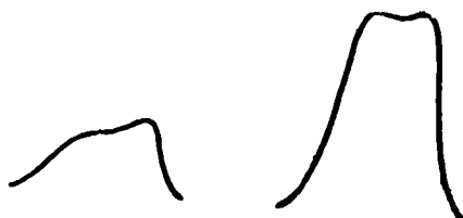
FIGS. 88 and 89.—On the left is seen the effect of heavy damping on an I.F. transformer, and on the right the result of removing the damping.
