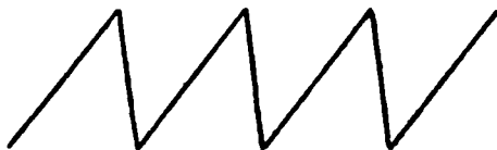
FIG. 80.—Saw-tooth waveform of voltage for X deflection as a function of time.
