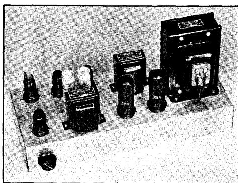
FIG. 1204 — METAL-TUBE SPEECH UNIT WITH PUSH-PULL 6L6 OUTPUT
