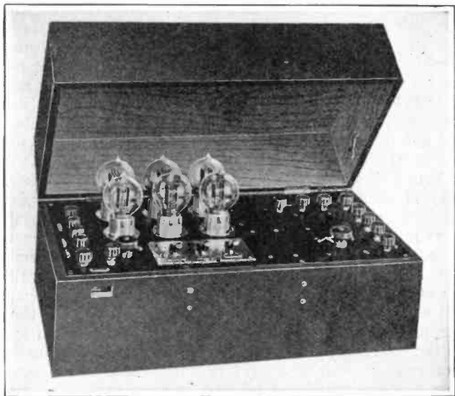
Special power amplifier, used in connection with extra powerful loud-speakers such as are employed for projecting the radio-phone entertainment in a large hall. This amplifier is used in addition to the usual amplifier of the receiving set.
