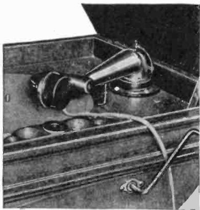
Loud-speaker attachment that fits on the tone-arm of any phonograph so that the usual horn of the phonograph is used to amplify the sounds.
