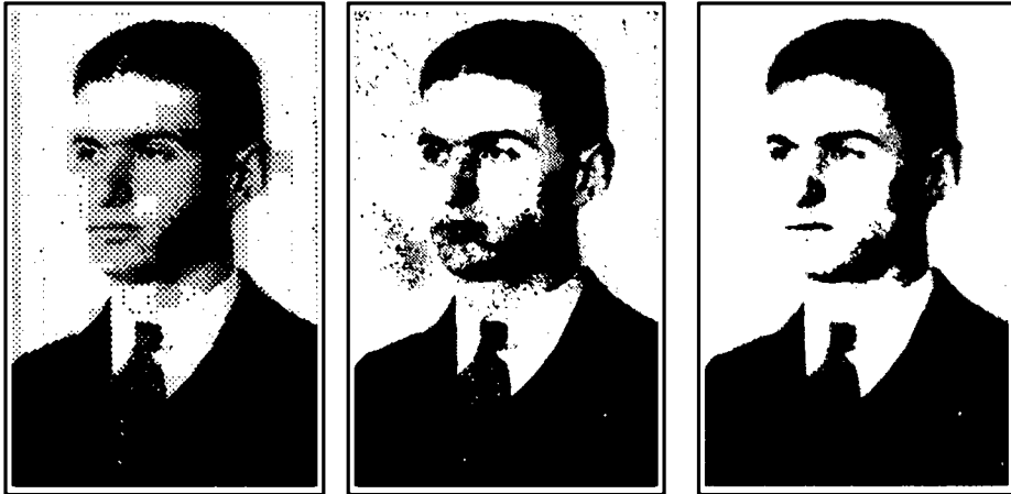
Fig. 447—The detail of the reproduced picture depends upon the number of picture elements used per unit area. At the left is a half-tone reproduction made up of individual dots of ink (picture elements) spaced 50 to the inch. There are 2,500 such elements per square inch in this. At the center is the same illustration made up of individual dots of ink spaced much closer i.e., 85 per inch. At the right there are 120 dots to the inch. Notice the poor detail of the picture at the left as compared to that on the right.
