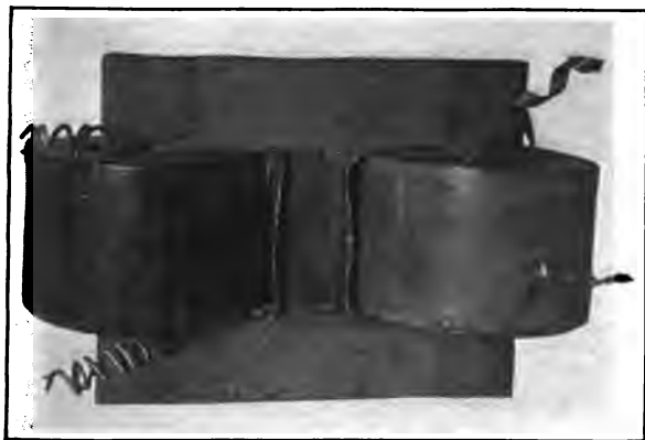
Fig. 18.—A Magnetic Leakage Transformer to Be Used on 110 Volts.
