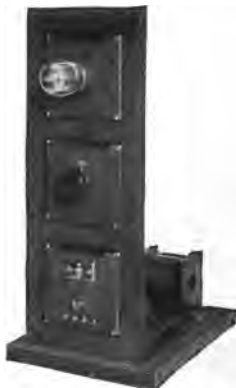
Fig. 79.—A Three Panel Audion Amplifier.
