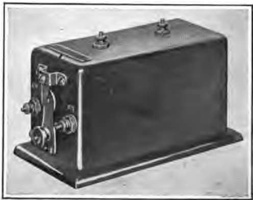
Fig. 8.—A Spark Coil for Small Transmitters.
