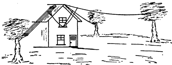
Fig. 35.—Antennas Are Provided for Transmitting, and Short and Long Wave Reception.
