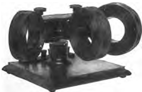
Fig. 53.—Two Handles Are Provided to Adjust the Position of the Outer Coils.
