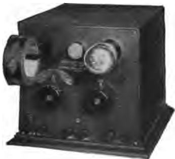
Fig. 50.—Here is a Complete Audion Receiver of the Simplest Type.
