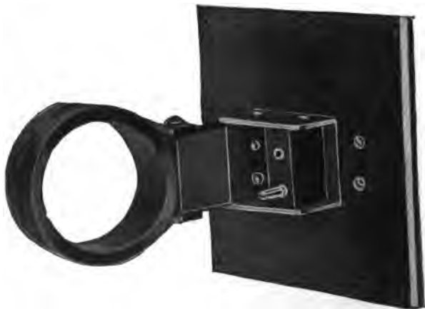
Fig. 38.—Two Coils Can Be Mounted in This Device for a Loose Amplifier.
