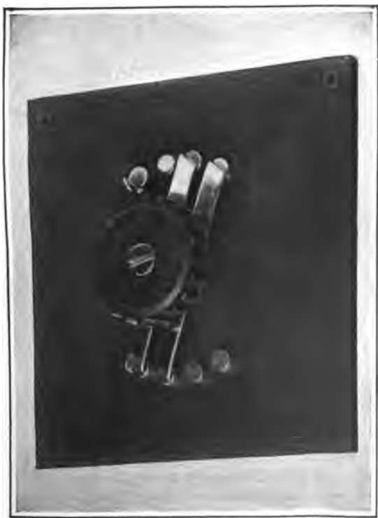
Fig. 57.—By Means of This Switch the Connections of the Condenser Can Be Changed.
