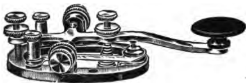
Fig. 12.—A Telegraph Key by Means of Which Dots and Dashes Are Sent.
