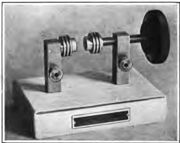
Fig. 15.—A Typical Construction for a Good Spark Gap.
