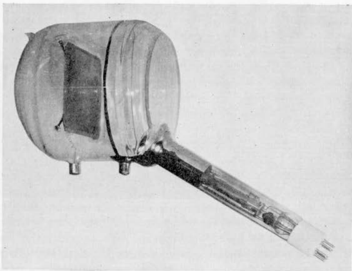
FIG. 125.—A form of iconoscope. The optical image passes through the flat glass window to the mosaic plate within the tube. The television signal is obtained from the two terminals at the bottom.
