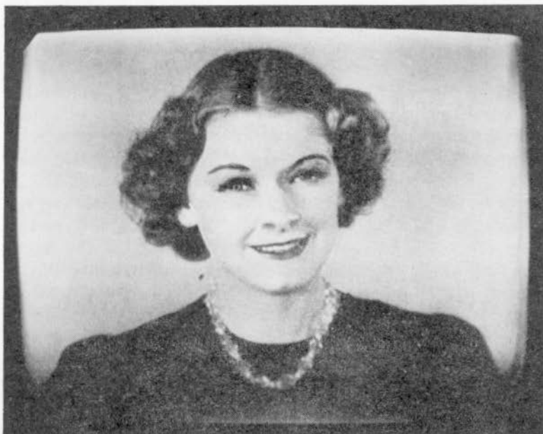
FIG. 126.—441-line television image, as it appears on the fluorescent screen of the cathode-ray receiving tube. (Photo taken in the experimental television studios of the National Broadcasting Company.)
