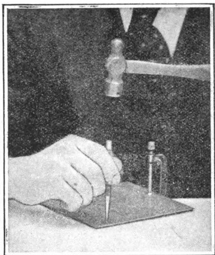
Fig. 29.—Using the jig for laying out a panel.
