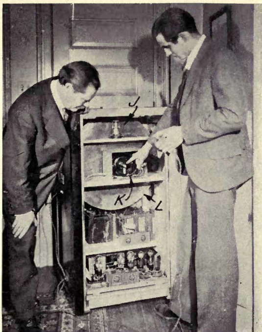
The inside of the Alexanderson television receiver. J points out the neon tube, K the synchronous motor and L the scanning disc. A powerful audio-frequency amplifier of special design is placed in the bottom of the cabinet.
