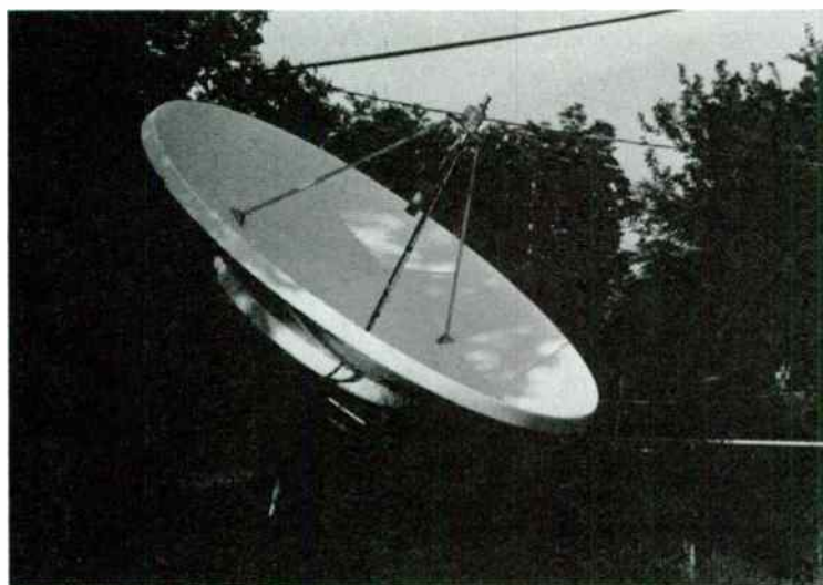
Fig. 10-17. A typical TVRO dish of fiberglass design performs extremely well with the Universal Communications system.
