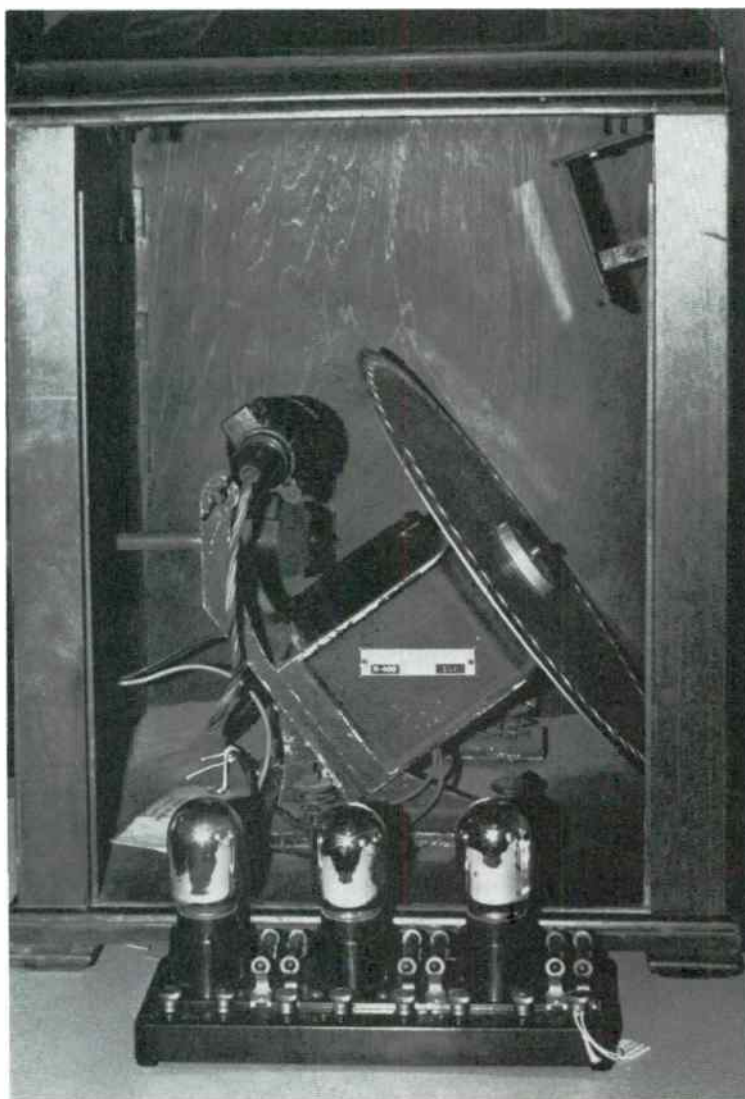
Fig. 2-4. Interior view of the Jenkins Radiovisor, showing Nipkow disc, mirror and amplifier section. This unit actually received pictures during the 1920s (courtesy W2BWK and ham radio magazine).
