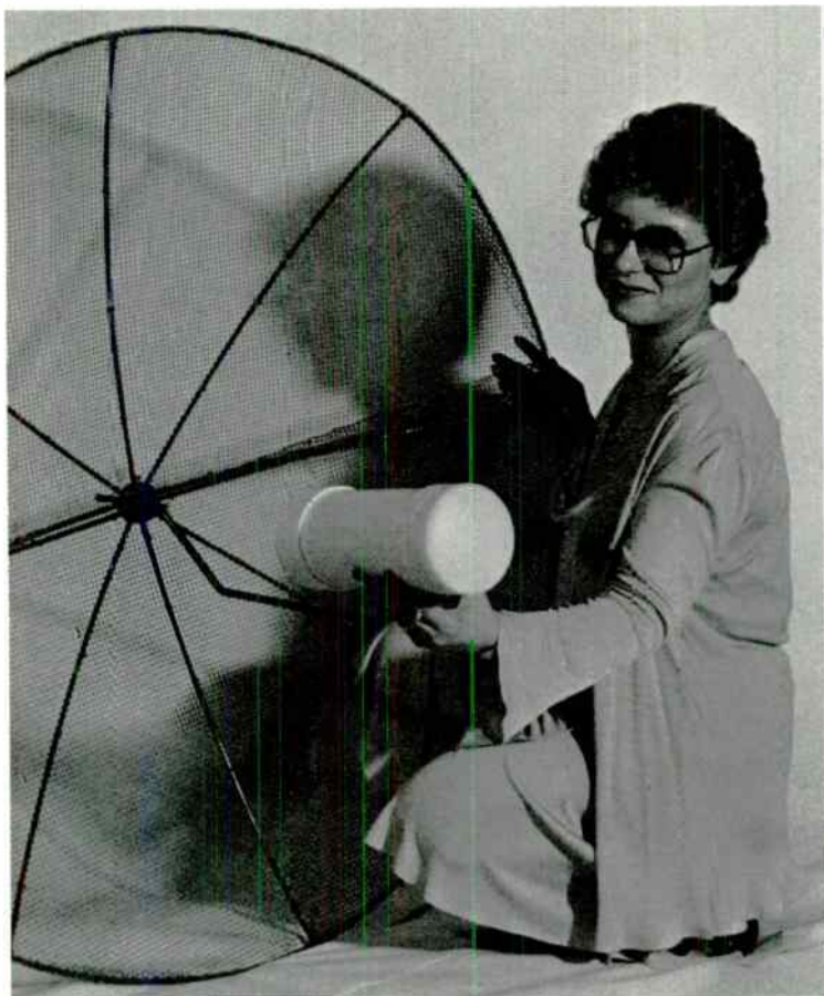
Fig. 9-13. Deborah with Universal Communications 4-foot parabolic dish and plastic enclosure for coffee-can cavity.
