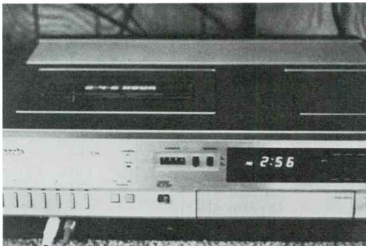
Fig. 12-8. This VHS recorder features vhf/uhf tuners with AFT and programmable timer.
