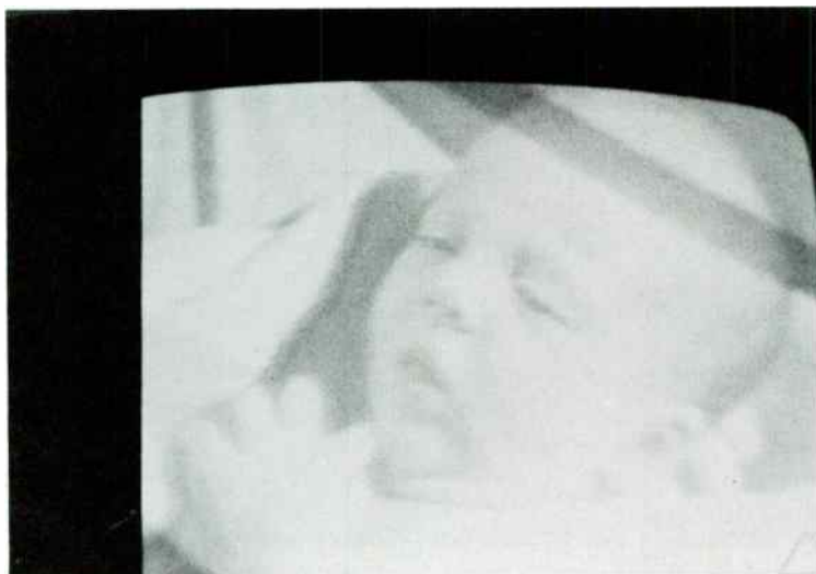
Fig. 14-5. Low contrast picture. Check settings of brightness, contrast, and agc. If problem persists, check video amplifier and video output stages.
