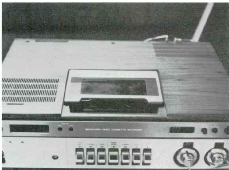
Fig. 1-7. This Betamax video recorder features internal vhf and uhf TV-tuner systems, permitting taping of movies independent of associated TV viewing.
