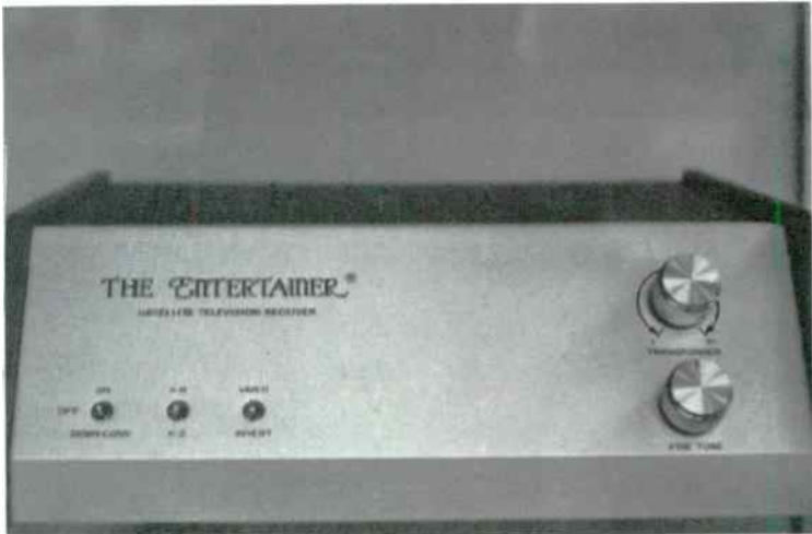
Fig. 1-4. One of a variety of indoor tuning units used with dish and LNA for satellite-TV reception.
