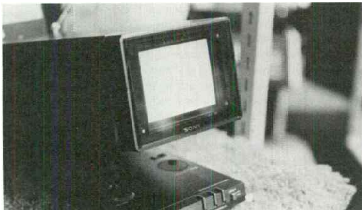
Fig. 1-11. This miniature color-television receiver features an on-screen tuning bar which moves left to right to indicate channels as they are tuned. The bar disappears five seconds after a channel is received.
