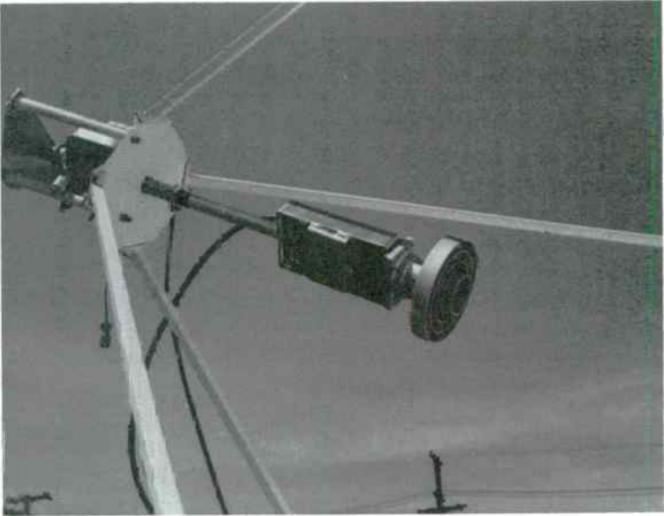
Fig. 1-3. A special unit, known as a low noise amplifier, is mounted at the focal point of the satellite TV dish and connected to the indoor unit via a coaxial cable. Note the circularly polarized waveguide on the front and the polarity rotor at the rear.
