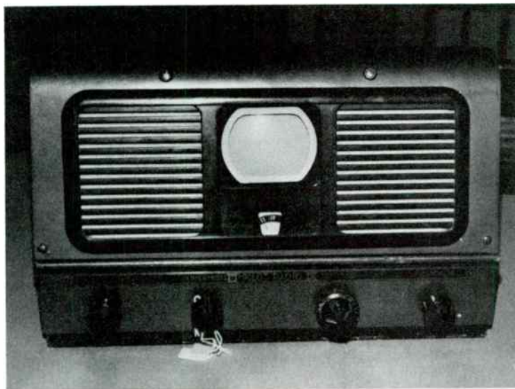
Fig. 2-6. This Pilot home-television set from the late 1930s was one of the first electronic-scanning sets offered to the public. Photo from Antique Wireless Association Museum (courtesy of W2BWK and ham radio magazine).
