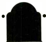
Fig. 4. This meter faceplate can be glued to any appropriate sized meter with a 5 mA full-scale rating.
