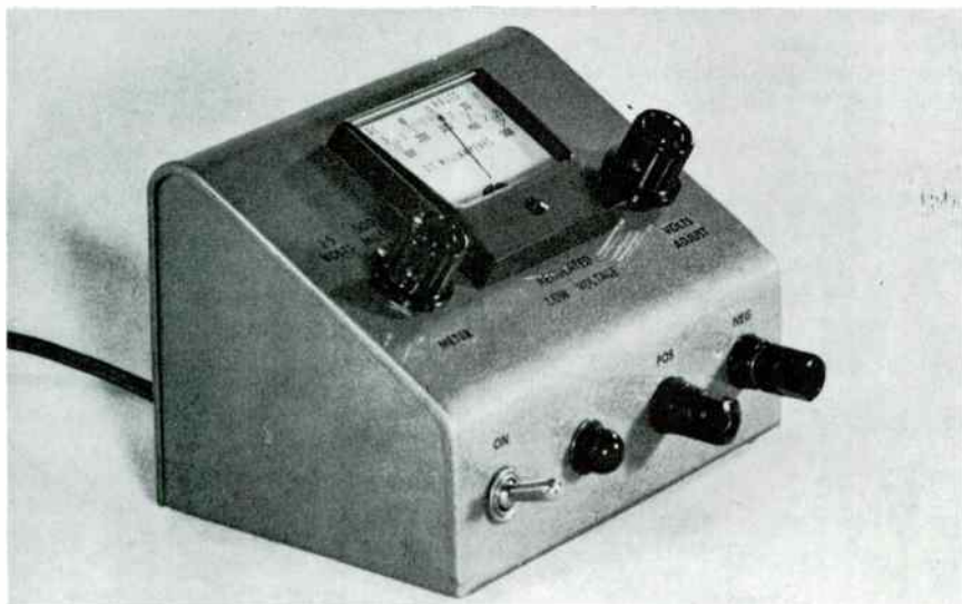
Exterior view of the 500 mA power supply. The case used is a Bud CMA 1930.
