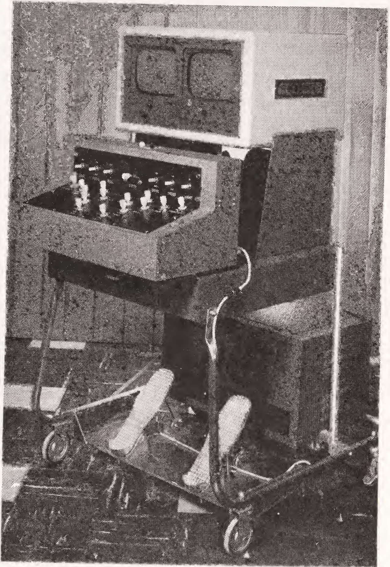
Fig. 7-5. A control panel for the Mobot Mark II. Courtesy Hughes Aircraft.
