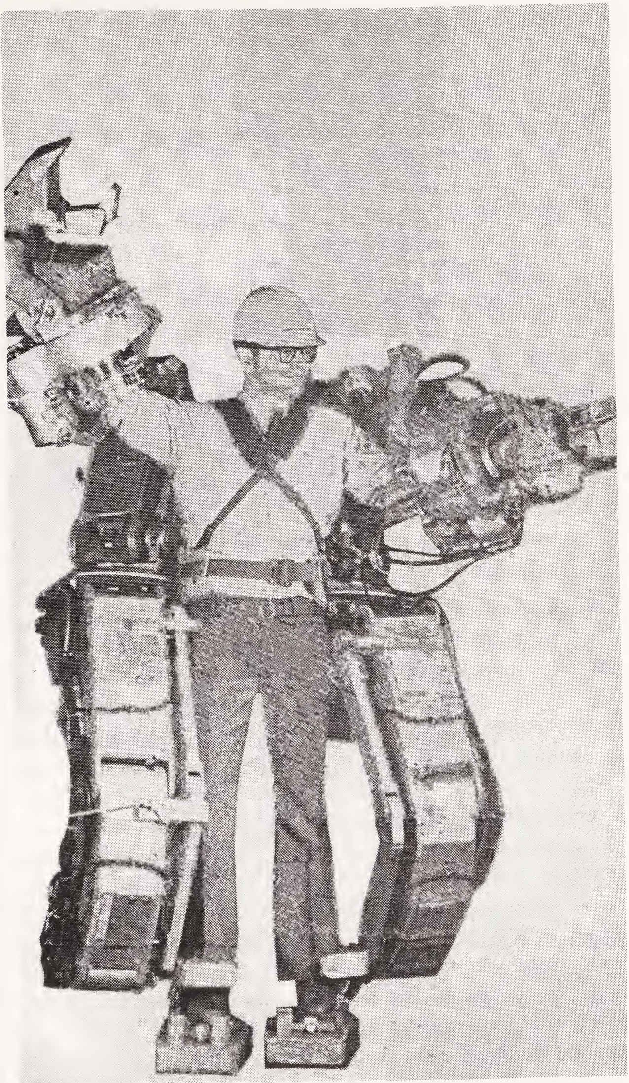
Fig. 9-7. Hardiman I, under human control and equilibrium, provides great strength. Courtesy General Electric.
