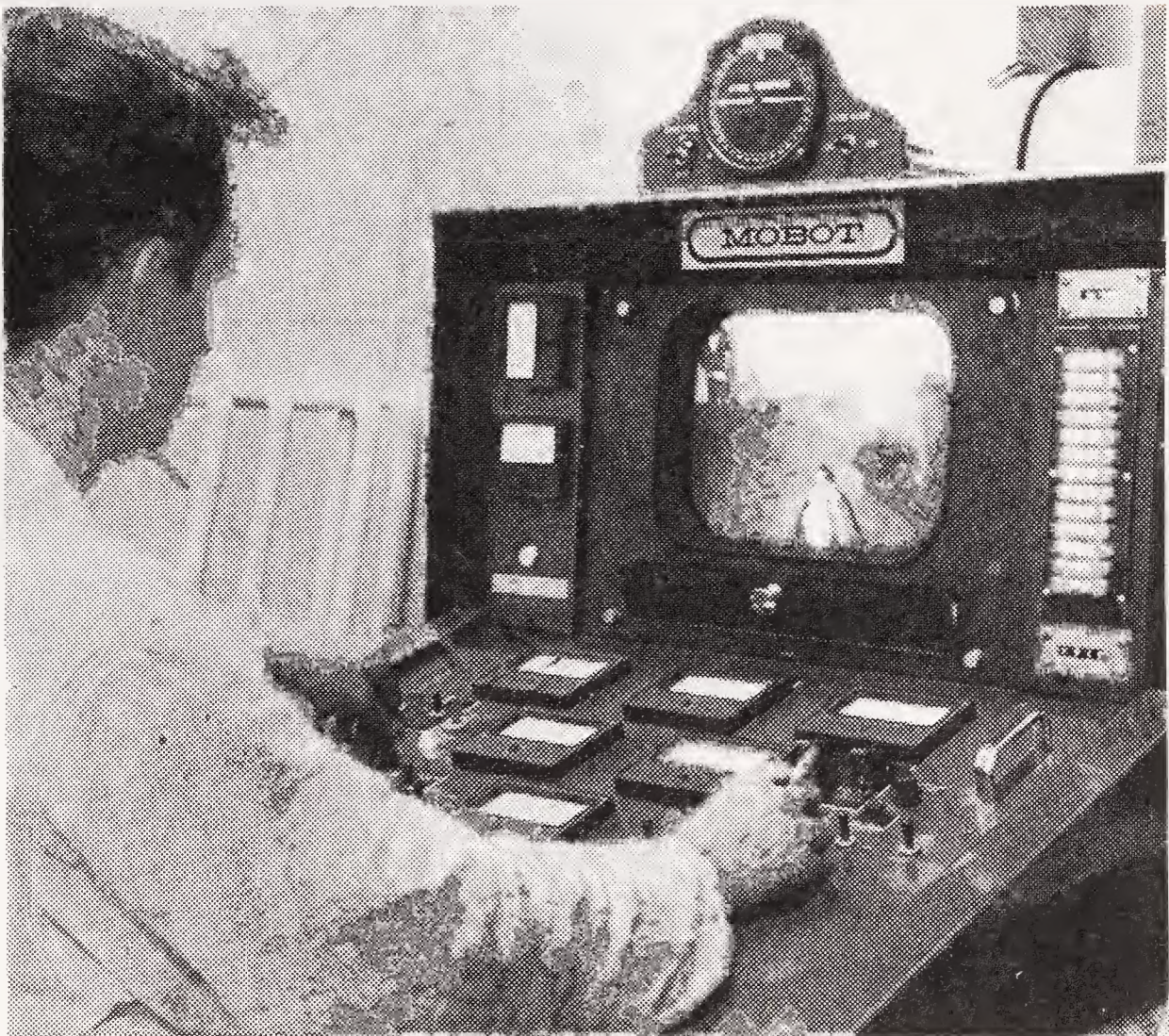
Fig. 9-2. A control panel for the Mobot. Courtesy Hughes Aircraft.
