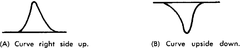
Fig. 3-9. Waveform aspect on scope depends on polarity of voltage at receiver output.
