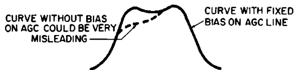
Fig. 3-18. Variation in IF-amplifier response due to change in AGC bias.
