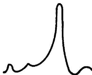
Fig. 8-2. A highly peaked bandpass-amplifier response curve.
