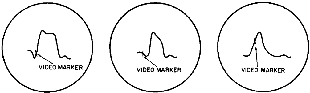
Fig. 4-10. Various video-IF response curves that might be encountered in a TV receiver.
