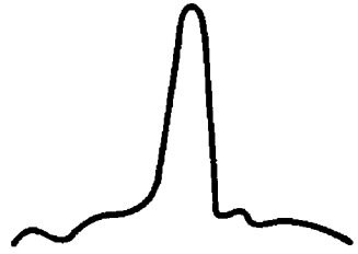
Fig. 8-5. A curve like this will result in transient irregularities in the reproduction of a color-bar signal.
