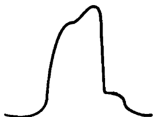
Fig. 8-1. IF response curve in an earlier color-television receiver.
