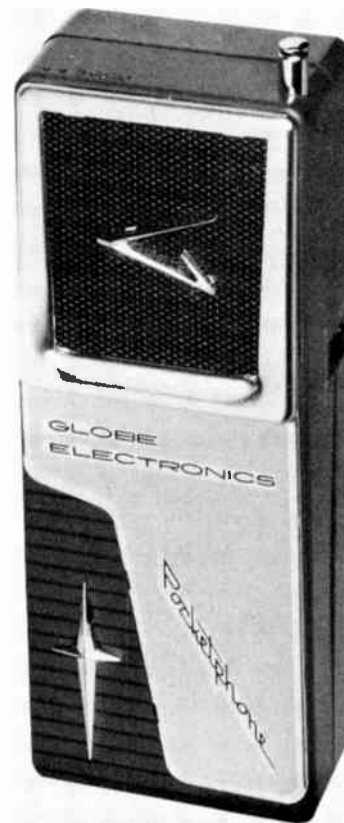
Fig. 11. Example of an all-transistor Class-D transceiver.
