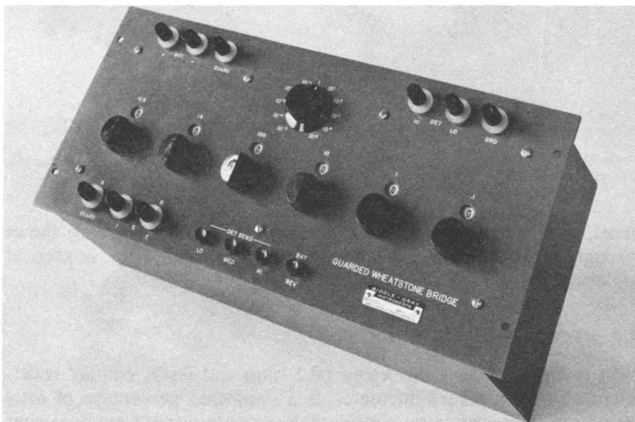
Fig. 2-10. Guarded Wheatstone bridge for close measurements.
