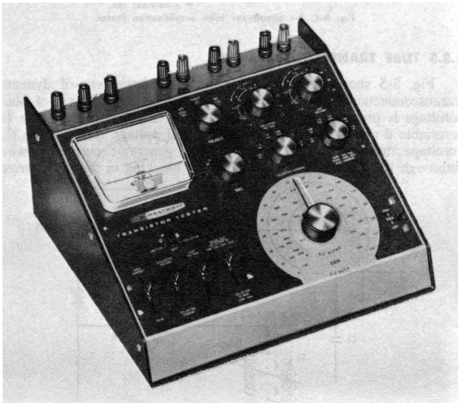
Fig. 8-6. Bridge-type transistor tester.
