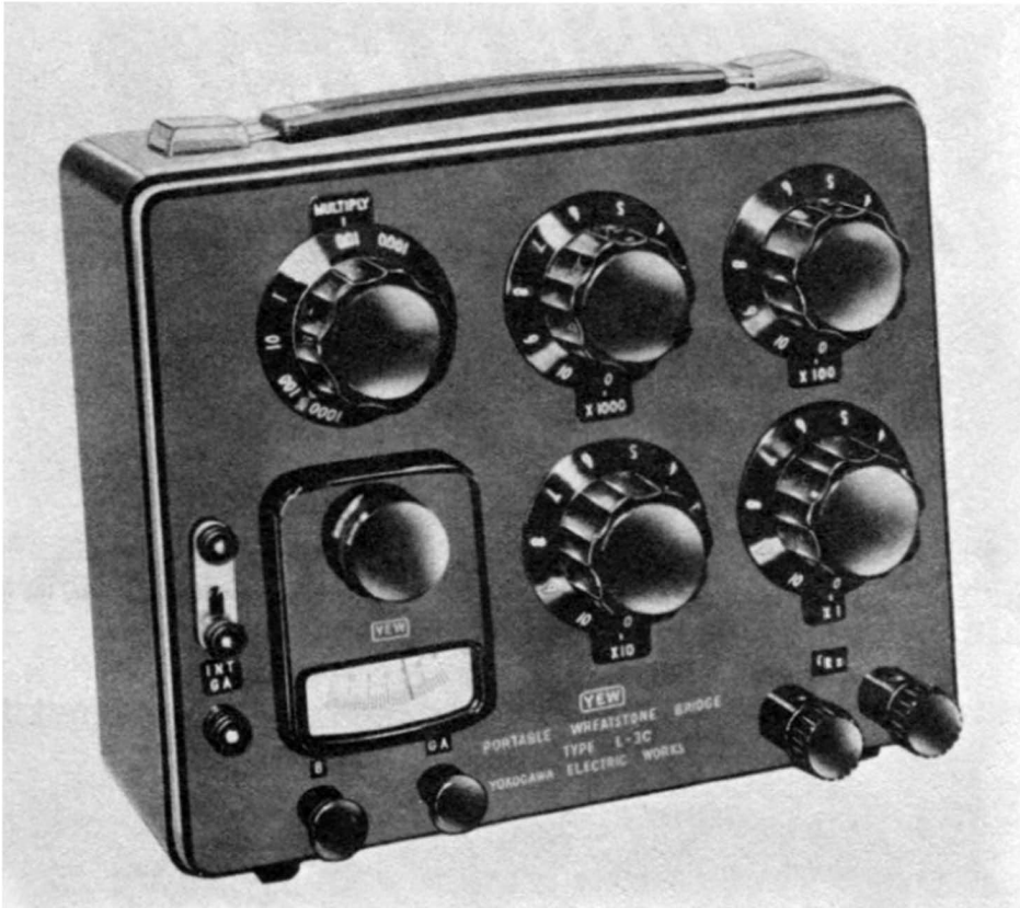
Fig. 2-8. Dial-type Wheatstone bridge.
