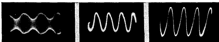
Fig. 229-A, left, Fig. 229-B, middle, Fig. 229-C, right. A. The wave envelope of the modulated output of a commercial test oscillator. B. The a-f. output of the same oscillator. C. The a-f. signal resulting from demodulation of the modulated wave shown in A.
