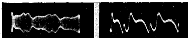
Fig. 236-A, left, Fig. 236-B, right. The same oscillator adjusted to 1000 kc. has a modulated waveform as shown in Fig. 236-A. The a-f. output resulting from the demodulation of A is shown in B.
