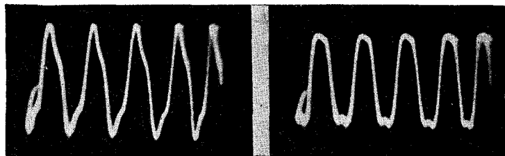
Figs. 165, left, 166, right. The composite wave of the waves shown in Figs. 163 and 164. Note the effect on the shape of the composite wave that a shift in phase has. See Fig. 166.
