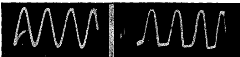
Figs. 213, left, 214, right. The waveform of the voltage across the secondary circuit is shown in Fig. 213. The waveshape of the voltage, showing cut-off, in the plate circuit of one of the sections of the 6A6 tube in the Class B stage.
