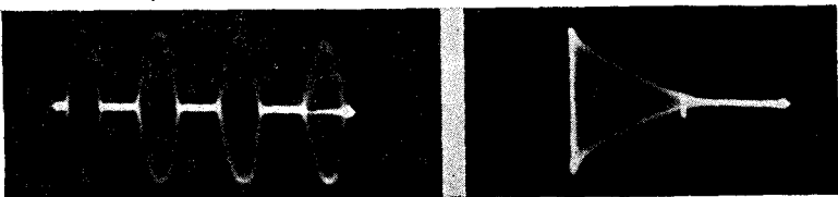
The wave envelope and trapezoid patterns are shown in Figs. 401 (left) and 402 (right). The trapezoidal patterns afford more definite information than is evident in the modulated wave pattern.
