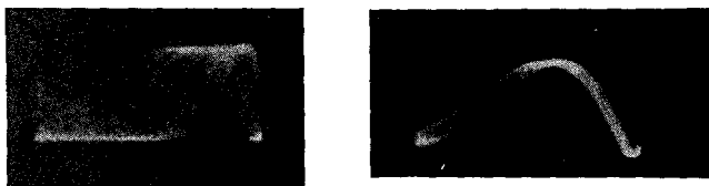
Fig. 71, left, Fig. 72, right. The pattern shown in Fig. 72 resulted from adjusting the synchronization control a trifle after the pattern in Fig. 71 was photographed. The pattern in Fig. 72 is still under-synchronized.
