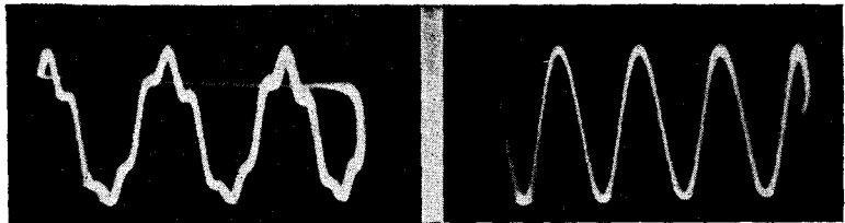
Fig. 239, left, Fig. 240, right. The oscillogram of Fig. 239 is the a-f. output of an oscillator with high L-C ratio and regeneration. The waveform of Fig. 240 is for the same oscillator when the L-C ratio and the regeneration were reduced.
