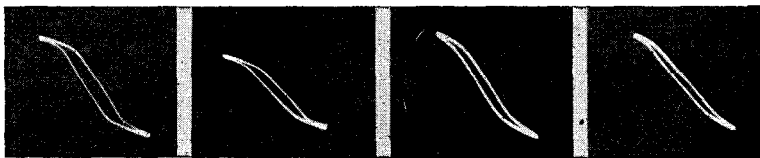
Figs. 142, 143, 144, 145 (reading from left to right). These hysteresis curves were made at 100 cycles. The greater the saturation, the flatter become the ends of the curve. Fig. 142 indicates the greatest saturation of these four oscillograms. Note that the area of these patterns (indicating the core loss due to hysteresis) is less than that of Fig. 147.
