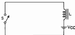
Figure 90. Simplest form of deflection circuit.
