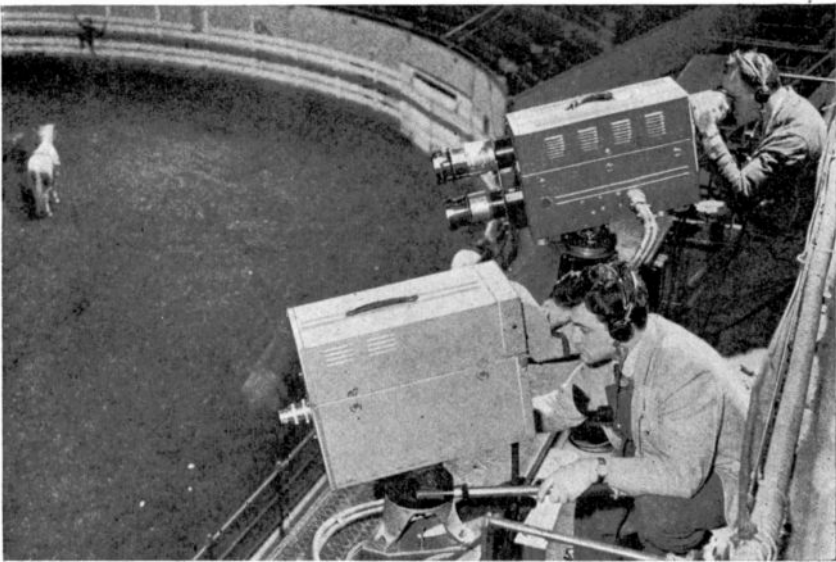
Fig. 9—Image Orthicon Camera (Foreground), in Comparative Test with Orthicon Camera, Televising Rodeo at Madison Square Garden.
