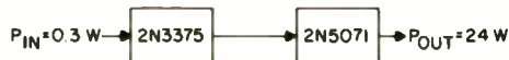
Block diagram of a 24-watt amplifier for 30-76 MHz operation. Schematic diagram available upon request.
