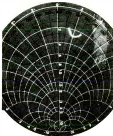
Fig. 11—Circuit-analyzer output-impedance trace for broadband amplifiers using output network shown in Fig. 10.
