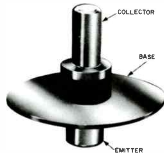
Fig. 1 - Specially designed, hermetically sealed, coaxial package for the 2N5470 rf power transistor.
