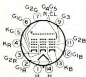
14AH ULTOR = G_4 + G_5 + CL + R FOCUSING ELECTRODE = G_3
