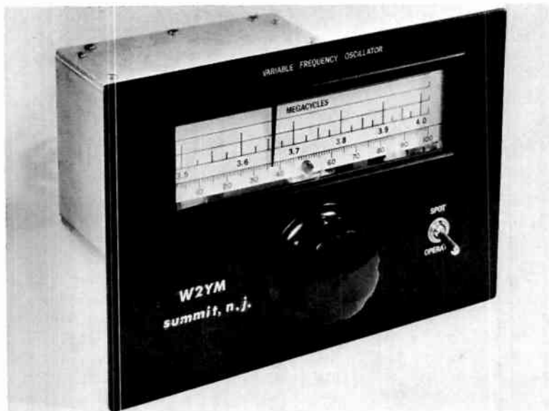
Fig. 159 - Suggested enclosure for the variable-frequency oscillator.
