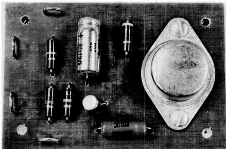
Fig. 130 - Completed circuit board for the electronic siren.
