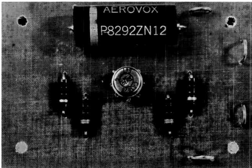
Fig. 63 - Completed circuit board for the simple code-practice oscillator.
