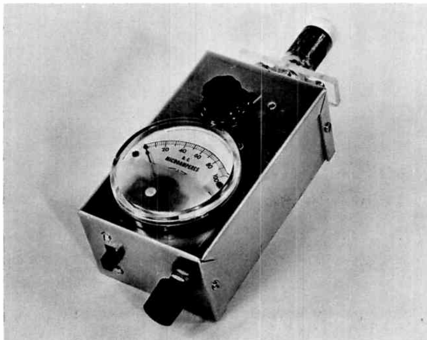
Fig. 156 - A suggested method of assembling the dip/wave meter.
