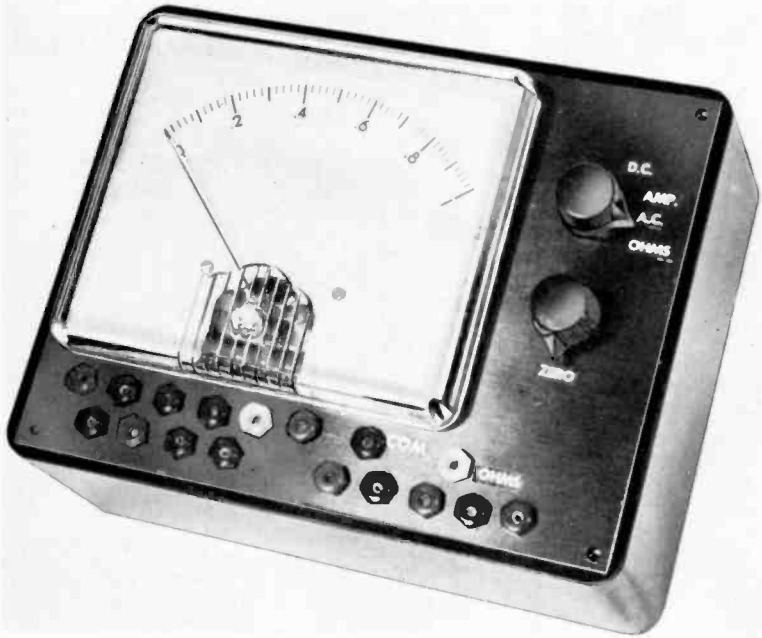
Fig. 309. This home-made unit was designed for a 50-microampere meter.
