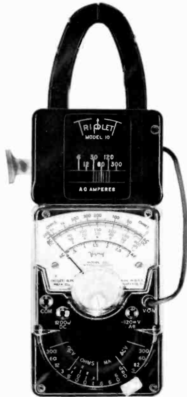
Fig. 503. Volt-ohm-milliammeter with a clamp-on transformer attachment. (Triplet Electrical Instruments Co.)
