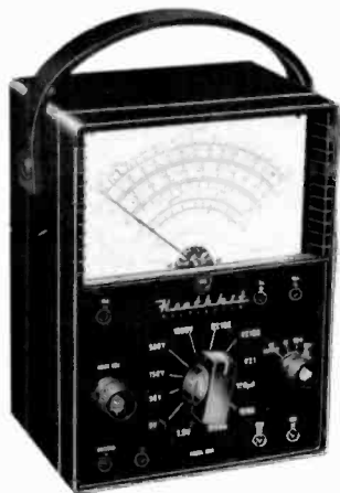
Fig. 403. Volt-ohm-milliammeter constructed from a kit. (Heath Co.)
