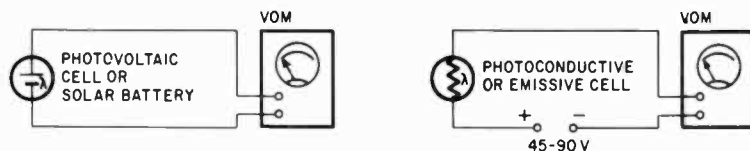
Fig. 1016. Simple photometric circuits using the vom.
