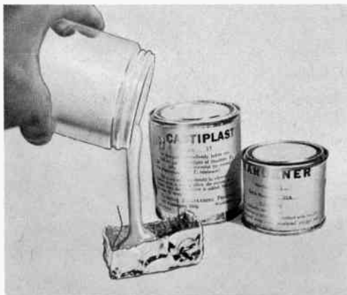
Fig. 655. The potting compound is poured around the component until it is covered.
