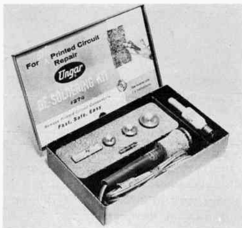
Fig. 518. Desoldering kit designed for use with printed circuits. (Courtesy Ungar Electric Co.)
