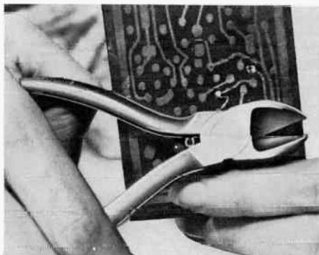
Fig. 510. Crushing the body of the component in the crotch of the pliers.
