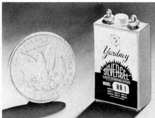
Fig. 408. A typical rechargeable silver-zinc battery. (Courtesy Yardney Laboratories.)
