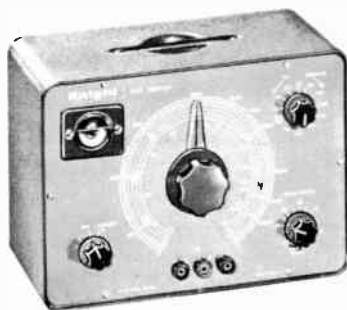
Fig. 524. Combined R-C bridge and in-circuit checker for servicing printed circuits. (Courtesy Allied Radio.)
