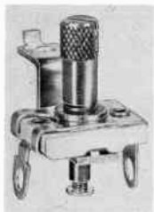
Fig. 325. Mica compression trimmers are easily adapted for miniature work; a) knob-tuned unit; b) shaft-tuned type. (Courtesy Arco.)
