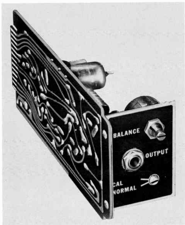
Fig. 108. A control unit used in conjunction with test instruments. The characteristics of a test setup are changed simply by substituting a different unit. (Swartwout Electronics Co.)
