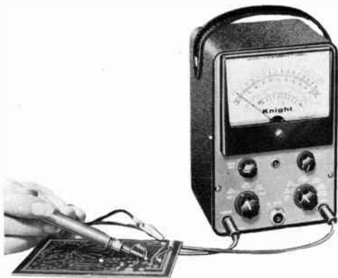
Fig. 502. Using a vtvm for point-to-point circuit checks. (Courtesy Allied Radio)
