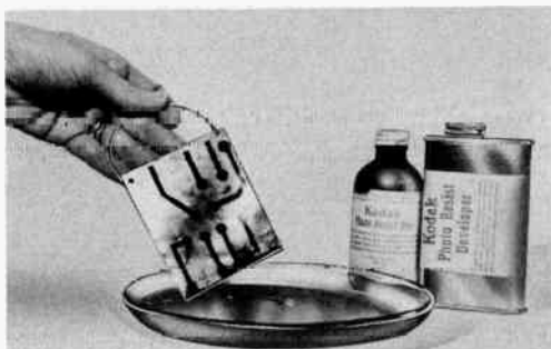
Fig. 208. Developing the exposed laminate plate.
