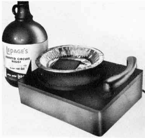
Fig. 209. A phono-turntable setup for whirling the plate when using the Permacel-Lepage glue-resist technique.
