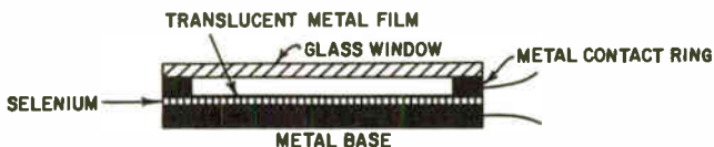
Fig. 810. Section of a selenium photovoltaic cell.
