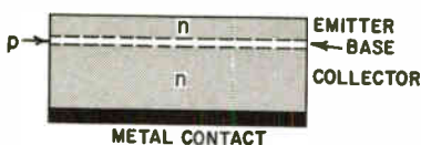
Fig. 714. The double-diffused technique enables transistors to be made with extremely thin bases.
