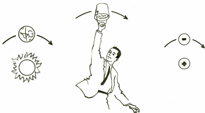
Fig. 207. Three examples of how things "stay up" in spite of attraction: (a) earth round sun, (b) water round man and (c) electron round nucleus.
