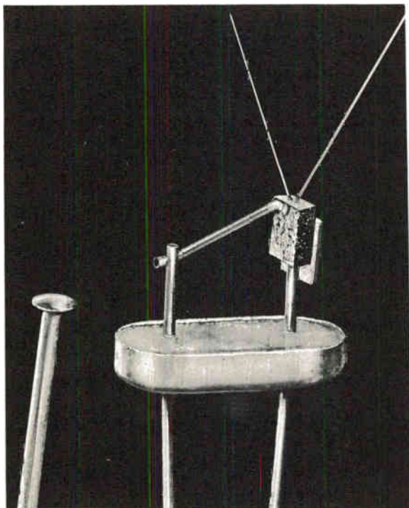
Fig. 718. Triode and tetrode varieties of the spacistor, another device that works on a different principle from the ordinary transistor. The photo shows the construction of a spacistor.
