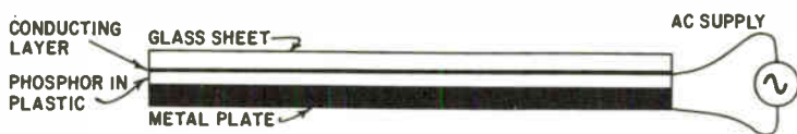
Fig. 907. Section of an electroluminescent panel, which glows under the stimulation of an alternating electric field.
