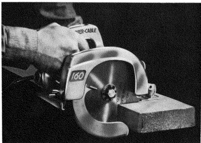
Fig. 604. The portable rotary saw can be used for cabinet work provided a suitable guide and the proper blade are obtained. (Courtesy Porter-Cable.)
