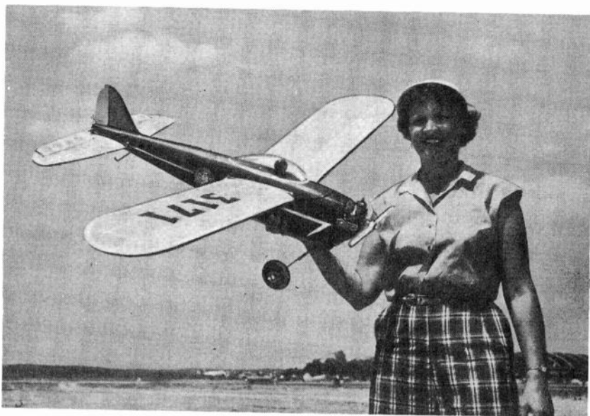
Fig. 1424. Author's wife holds shoulder wing "Kickin' Duck" plane. Though much overweight, it was good performer. All low-voltage requirements of the plane, including receiver filament supply, were handled by a single LR-1 Silver-cel. This arrangement was used in effort to keep weight down.
