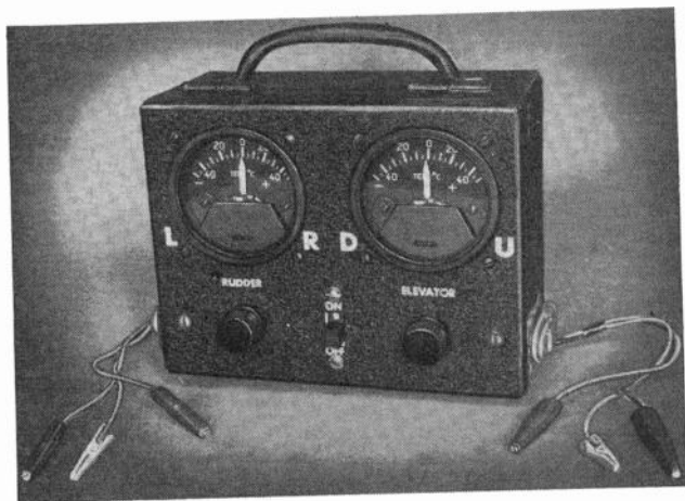
Fig. 1321. This pulse tester used surplus meters, is mounted in surplus meter case. Actual scale reading is of no consequence, but it must be the same both sides of center.
