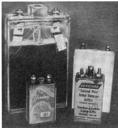
Fig. 902. Plastic-cased alkaline cells include surplus nickel-cadmium 5 ah (ampere-hour) unit at left rear (popular in transmitters and for engine starting), the ABC (also known as CG or Gulton) VO-800 at right rear; left front is Yardney LR 1 Silvercel, and at right, the Sonotone 1 ah nickel-cadmium battery.
