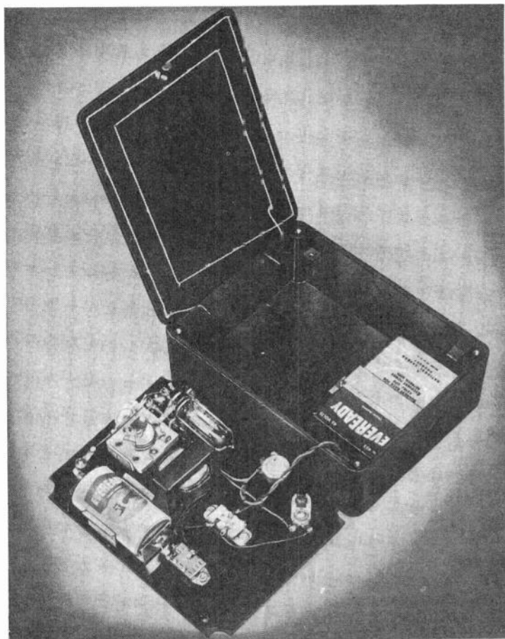
Fig. 1311. Simple 27 mc direction finder with panel out of case. Due to size of case, subminiature parts are not required and over-all cost is low. B-battery gives very long life; A-battery will be as good, if recommended mercury cell is used. If not, the "alkaline energizer" type of dry cell is best.
