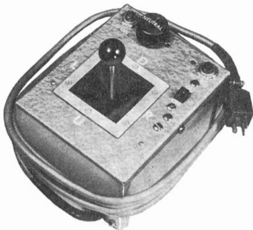
Fig. 822. The "compact" pulser, so-called because all batteries are in 3 x 4 x 5" case. Large knob at case upper edge is rudder trim control.
