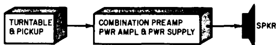
Fig. 401. The simplest form of a single-channel high-fidelity system contains just three components: the record player, the preamp-amplifier combination and the speaker system. For many installations, this is all that will be required.
