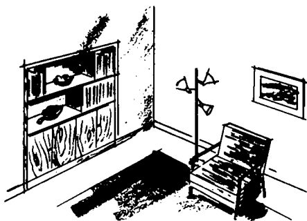
Fig. 1108. Built-in installation sunk into a wall.
