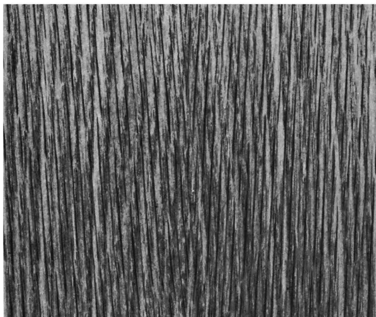
Fig. 1207. The even grain lines of comb-grain oak make it a very popular wood for furniture. (Hardwood Plywood Institute.)
