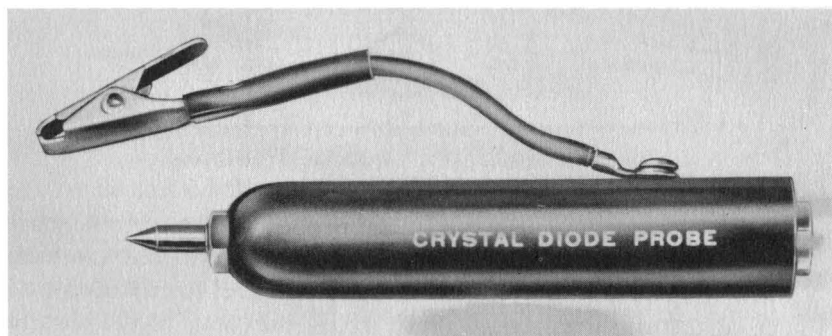
Fig. 407. Crystal-diode probe. The ground clip should be fastened as close to the test point as possible.
