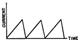
Fig. 606—Saw-tooth wave shape of current in deflection yoke.
