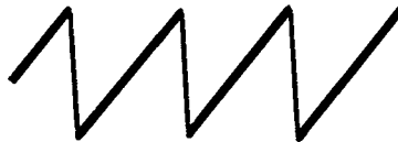
Fig. 605—Saw tooth as it should appear on the c.r.o. screen. The flyback lines should be very faint. The zero line (X-axis) should not be visible at all. The ends of the teeth should not be rounded off.
