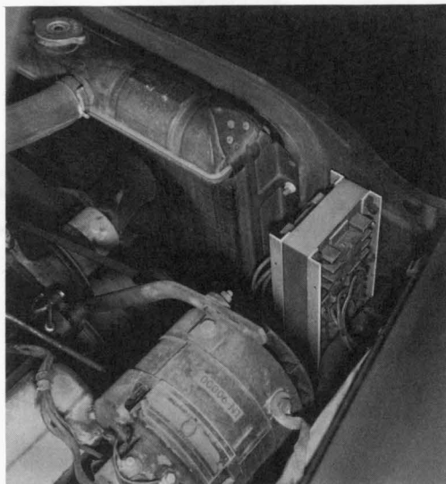
ENGINE COMPARTMENT VIEW of W8DLD's station wagon, showing Leece-Neve alternator in foreground and 3-phase distribution transformer mounted just ahead of it next to radiator.
