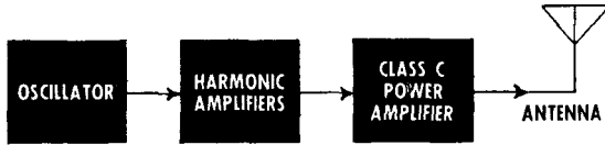
Fig. 1. Block diagram of a typical multi-stage transmitter to which a CW or AM system may be connected.
