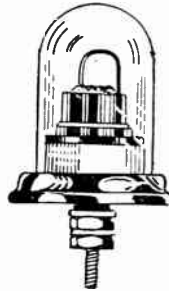
FIG. 4.—Crystal Detector with Fixed Cat Whisker.
