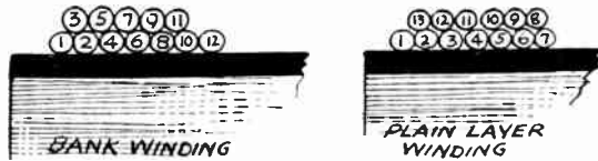
FIG. 1.—Bank Winding of Two-Layer Coil.
