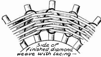
FIG. 3.—Lacing the Finished Diamond Weave Spiderweb Coil.
