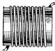
Space Winding on Single Layer Coil.
