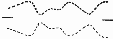
FIG. 4.—The Envelope of the Modulated Carrier.
